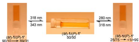
Figure 4. Photographs of the gel (3 mg/mL in \text{CH}_2\text{Cl}_2 ) at ambient temperature after irradiation of the original ( M )-1-containing gel at 318 nm for at least 60 min (middle) and then at 280 nm (right) or 343 nm (left) for another 6–8 h.
